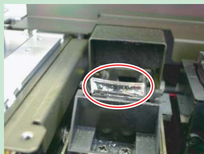
The example of deformed wiper
